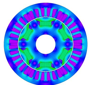
**Figure 1:** Model of a permanent magnet synchronous motor.
