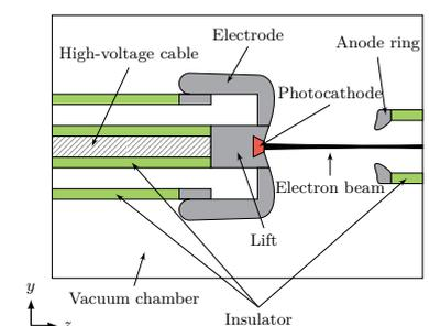
**Figure 1:** Schematic design of an electron gun.
